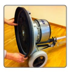
3) Raise the handle to an upright position, pull out the front carry handle and fold the handle shaft.
