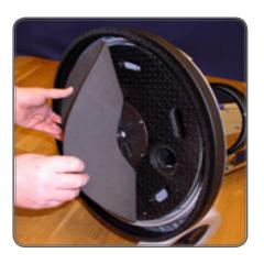
4) Insert and tighten the centre screw. NOTE! Tighten counter clockwise!
