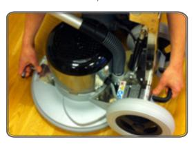
NOTE! Always remove the dust skirt and the sanding disc before transportation!
